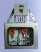
Designed for use in Zone 1 or Zone 2 hazardous areas, the air aspirated system uses a compressed air driven vacuum generator to draw a gas sample from a single point. Explosion-proof gas detectors are fitted to monitor for flammable gases, toxic gases or oxygen. Each detector provides a 4-20mA output. An intrinsically safe flow-fail device warns if the sample flow is lost due to supply air failure or sample line blockage.
